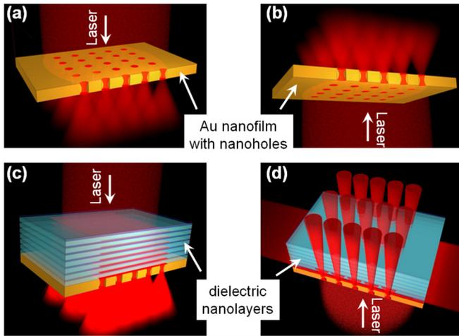
FIG. 9. (Color online) Scheme of experiments on measuring the asymmetry of light transmission with a perforated metal film: (a),(b) Light transmission through the perforated metal without the photonic crystal; (c),(d) light transmission through the perforated metal film on the photonic crystal where asymmetry of the light transmission is expected.
