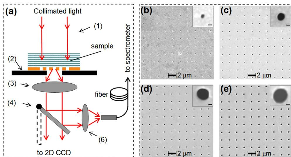
FIG. 10. (Color online) (a) The experimental setup to investigate the asymmetry of light transmission; (b)–(e) electron-microscope images of the samples under investigation with nanohole diameters of 100 (b), 200 (c), 300 (d), and 400 (e) nm. The insets of panels (b)–(e) show enlarged electron-microscope images of the individual nanoholes that form the corresponding perforated gold nanofilms (the length of the bar in the inset corresponds to 100 nm).
