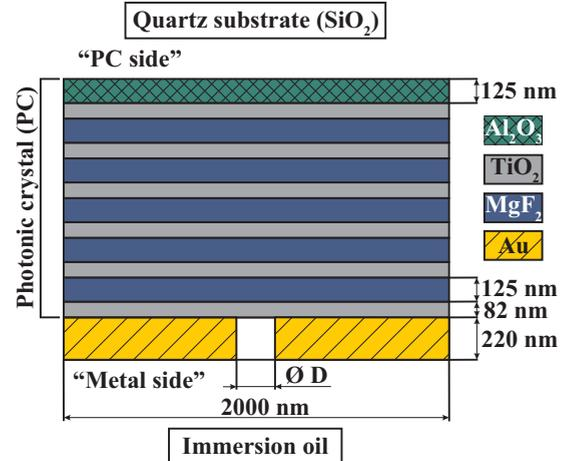
FIG. 2. (Color online) Schematic image of one period of a square lattice of circular nanoholes with a period of 2000 nm.
