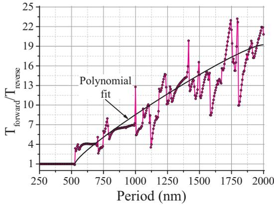
FIG. 6. (Color online) The light asymmetry coefficient ( $\xi = T_{\text{forward}}/T_{\text{reverse}}$ ) as a function of the period of the square lattice of nanoholes in the metal film. The diameter of the nanohole is 150 nm. The wavelength of the incident light is 796 nm.
