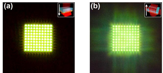
FIG. 12. (Color online) Manifestation of the asymmetry of light transmission of the perforated gold nanofilm on the photonic crystal under illumination with white light. The figure shows the optical images of the surface upon its irradiation from (a) the photonic crystal and (b) the metal film. In the insets the white arrows show the light beam direction.
