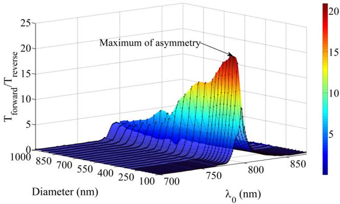
FIG. 3. (Color online) Ratio between the transmission coefficients upon incidence of light from the side of the photonic crystal ( $T_{\text{forward}}$ ) and from the side of the metal film ( $T_{\text{reverse}}$ ) in relation to the wavelength of the incident light and the hole diameter. The period of the structure is 2000 nm.
