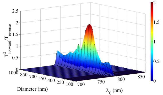
FIG. 7. (Color online) Figures of merit of our optical diodelike system,  $\eta = (T_{\text{forward}}/T_{\text{reverse}})T_{\text{forward}}$ . The period of the system is 2000 nm.
