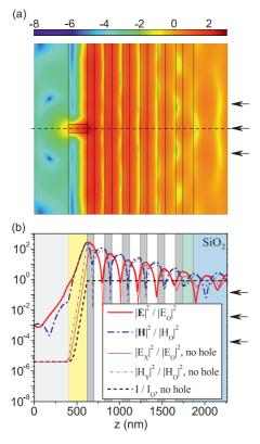
FIG. 6. (Color online) (a) Distribution of the electromagnetic field  $(|\mathbf{E}|^2/|\mathbf{E}_0|^2)$  of a plane light wave propagating through the optical structure metamaterial–metal-film with apertures in the case where the light wave is incident on the structure from the side of the metamaterial at resonance ( $\lambda=796$  nm). (b) The section of the two-dimensional distribution (a) along the dashed line. A logarithmic scale is used.
