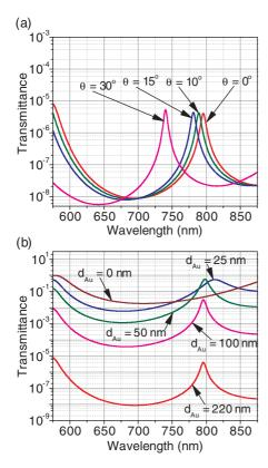
FIG. 3. (Color online) Dependencies of the light transmission coefficients through the optical structure metamaterial–metal-film: (a) on the wavelength and on the angle of incidence of light; (b) on the wavelength and on the thickness of Au film  $(d_{Au})$  for normal incidence of light.
