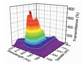
FIG. 7. (Color online) Dependencies of the transmission coefficient through the optical structure metamaterial–metal-film with apertures on the wavelength of the incident light for different sizes of apertures (the light is incident from the side of the metamaterial and we use the normalization to the light flux incident on the aperture cross section). Experimental data (100 nm) correspond to left side of the plot.
