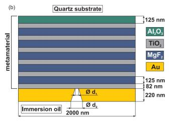
FIG. 1. (Color online) (a) Images of the array and one of the nanoapertures in the experiment of [10] obtained by the scanning electron microscopy method; (b) schematic image of the cross section of one period of the nanoaperture array in the gold film on the metamaterial used in the numerical experiment.
