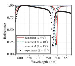
FIG. 2. (Color online) Dependencies of the reflection coefficient on the wavelength and on the angle of incidence of light for the optical structure metamaterial—metal-film.
