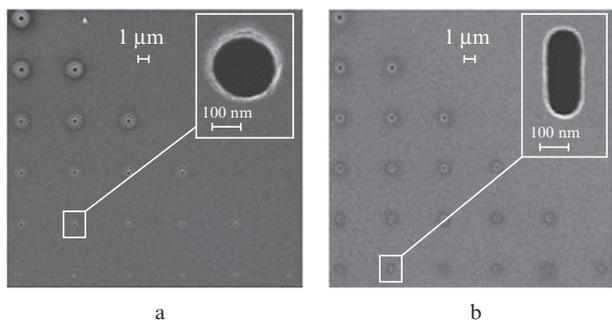
**Figure 2.** Nanohole images of (a) circular and (b) slit-like form in the aluminium film with the thickness of 50 nm, obtained by an electron raster microscope. Enlarged images are shown in the insets.
