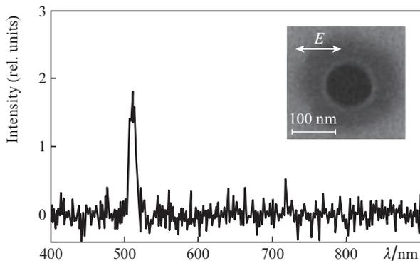
**Figure 3.** Radiation spectrum of the single nanohole in an Al film excited by the femtosecond laser radiation at the wavelength of 1560 nm. The hole image obtained by electron microscope is shown in the inset. Here and in Figs 5 and 6 the arrow denotes the electric field direction of exciting radiation.
