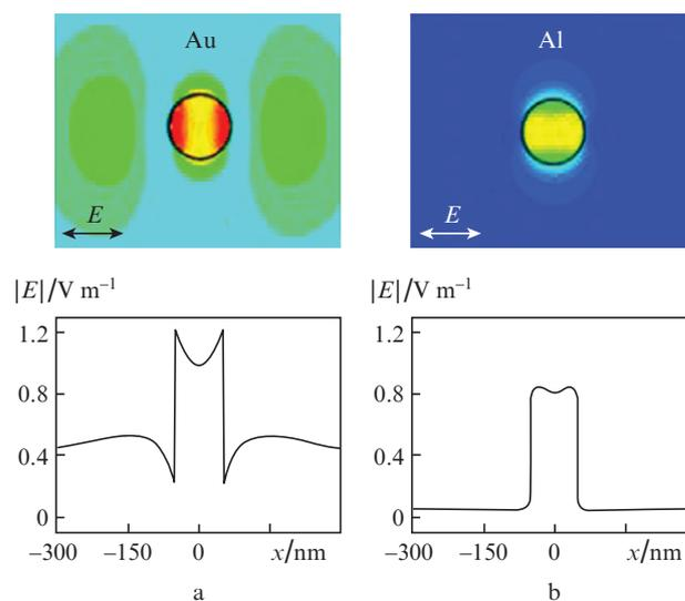
**Figure 5.** Calculated spatial distributions of the electric field amplitude at the wavelength of 520 nm near the hole with the diameter of 100 nm in 50-nm-thick (a) gold and (b) aluminium films.
