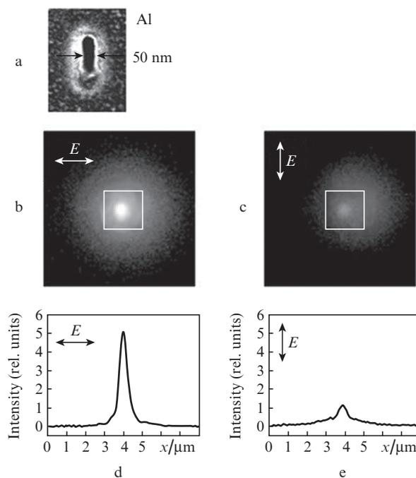
**Figure 6.** THG on the nanoslit of size  $50 \times 170\ \text{nm}$  made in the  $50\text{-nm}$ -thick aluminium film. (a) The slit image obtained by the electron microscope and the image at the third harmonic wavelength obtained by an optical microscope when the polarisation of exciting radiation is per (b) parallel to the slit axis; panels (d) and (e) show the corresponding intensity distributions.
