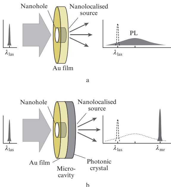
**Figure 7.** (a) Scheme of nanocalibrated and wideband radiation sources based on metal PL, and (b) scheme of similar source with photonic crystal.
