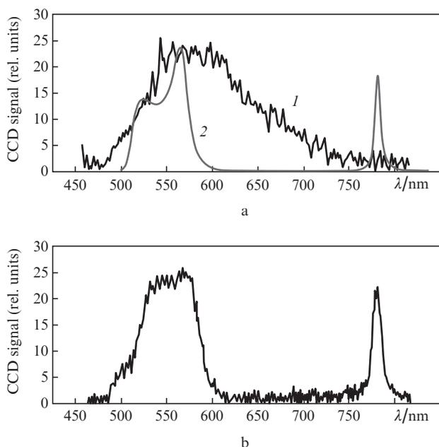
**Figure 10.** (a) PL spectrum of a nanohole with a diameter of 60 nm in a 200-nm-thick gold film (1) and calculated transmission spectrum for the nanohole in a microcavity (2) as well as (b) measured emission spectrum of a nanohole in a microcavity [34].
