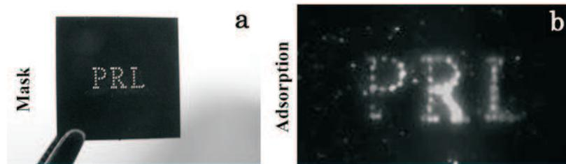
Fig. 6. (a) The mask consists of 35 holes in a thin metal foil. (b) The microstructure of Rb atoms in the form of three letters P R L that are obtained by the laser induced quantum adsorption.
