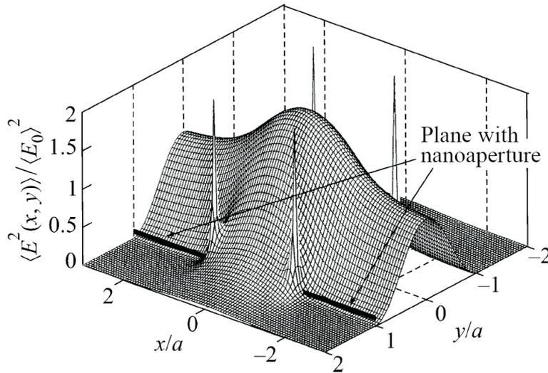
Fig. 2. Electromagnetic-field intensity for a photon hole.
