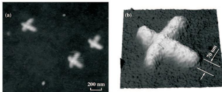
Fig. 4. Nanostuctures of Cr atoms on the glass surface that are obtained using the pinhole camera and the "cross" atomic object. Surface sections of sizes (a)  $2 \times 2 \mu\text{m}$  and (b)  $800 \times 800 \text{ nm}$  are shown. The nanostructures are measured by means of an atomic force microscope.
