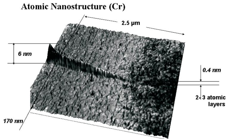
Fig. 3. Nanostructure of Cr atoms built with the atom nanopencil.
