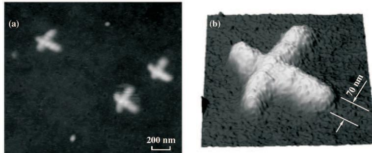
Fig. 4. Nanostructures of Cr atoms on the glass surface that are obtained using the pinhole camera and the "cross" atomic object. Surface sections of sizes (a)  $2 \times 2 \mu\text{m}$  and (b)  $800 \times 800 \text{ nm}$  are shown. The nanostructures are measured by means of an atomic force microscope.
