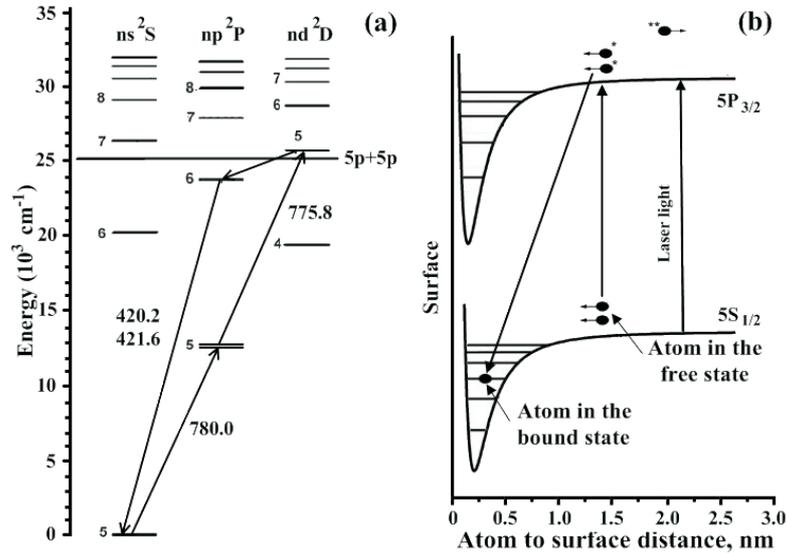
Fig. 5. (a) The energy level diagram for Rb atom. (b) The mechanism of loading of Rb atom in the surface trap.
