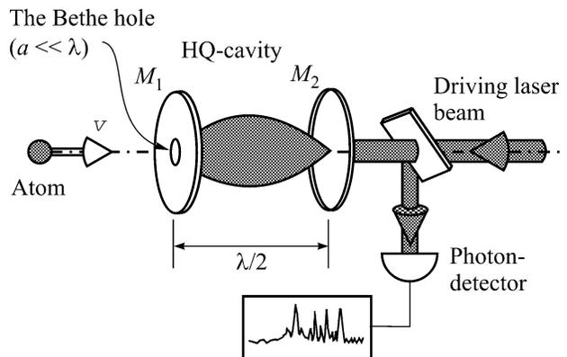
Fig. 1. Layout of an atom nanoprobe.
