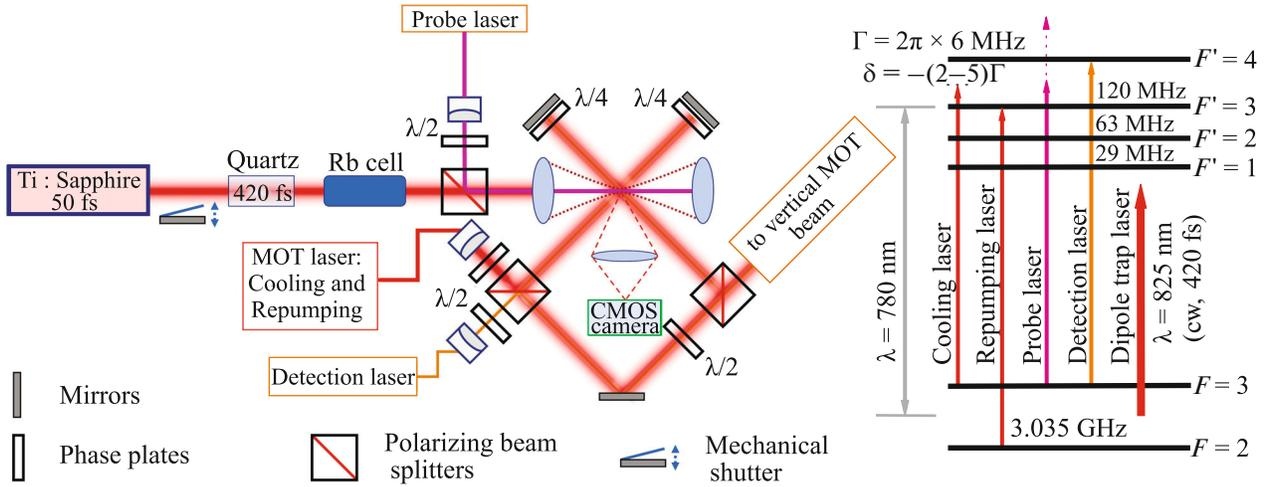
Fig. 1. (Color online) Experimental setup for studying the spectral properties of atoms localized in a pulsed dipole trap.
