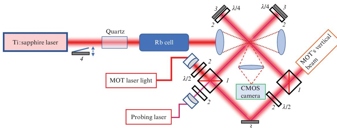
**Figure 3.** Schematic of the experimental setup used to study the effect of spectrally selective light filtering on the lifetime of atoms in a pulsed optical trap: (1) polarising beam splitter, (2) phase plate, (3) mirror, (4) mechanical shutter.
