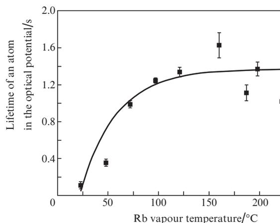
**Figure 4.** Effect of the rubidium atomic vapour cell temperature on the lifetime of atoms localised in the optical potential produced by pulsed laser light.
