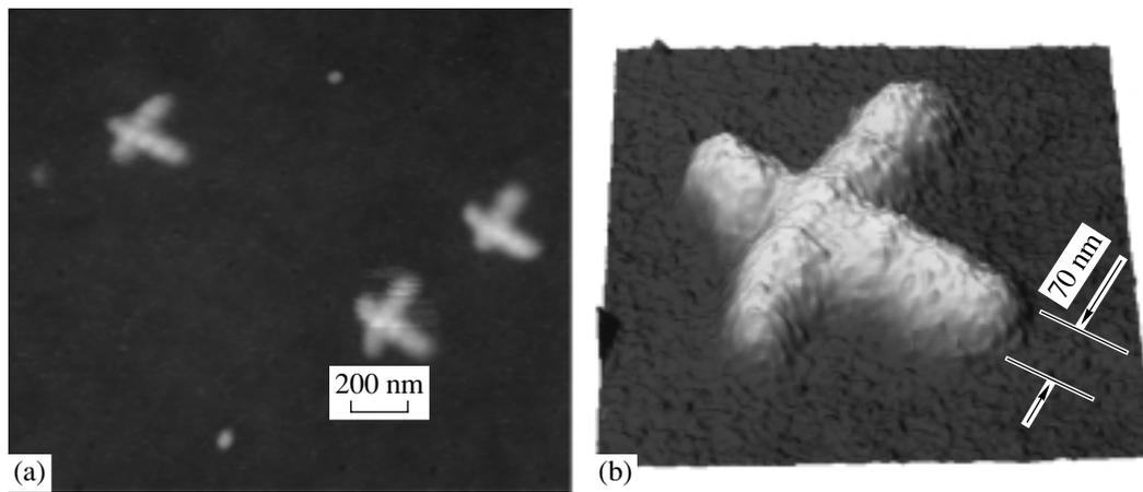
**Fig. 3.** Nanostructures formed of Cr atoms on the glass surface, obtained with an atomic obscure camera and an object mask in the form of a cross. Substrate portions with areas of (a)  $2 \times 2 \mu\text{m}$  and (b)  $800 \times 800 \text{ nm}$  are shown.
