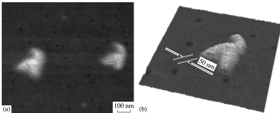
**Fig. 4.** Nanostructures formed of Cr atoms on the glass surface, obtained with an atomic obscure camera and an object mask in the form of the Greek letter  $\lambda$ . Substrate portions with areas of (a)  $1 \times 1 \mu\text{m}$  and (b)  $500 \times 500 \text{ nm}$  are shown.
