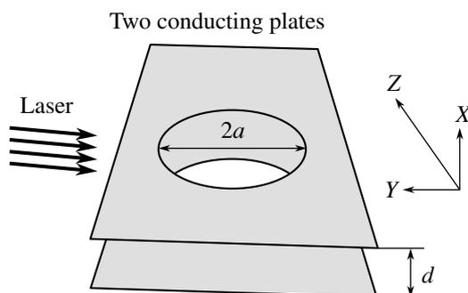
**Fig. 1.** Schematic diagram of formation of a spatially localized light nanofield serving as an atomic lens. Two planar conducting plates, spaced by a distance on the same order of magnitude or smaller than the light wavelength, form a two-dimensional waveguide for the laser radiation introduced into it from aside.
