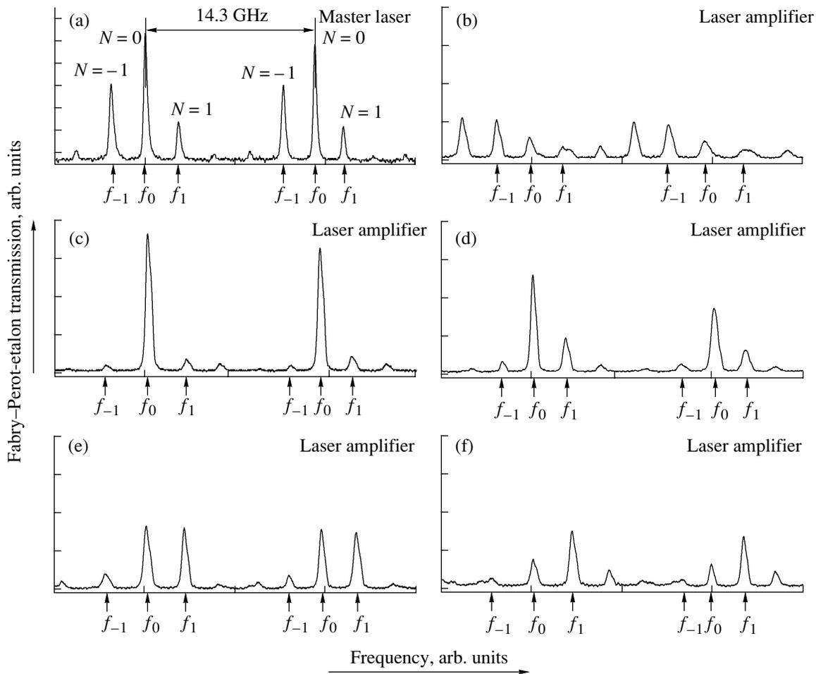
**Fig. 5.** (a) Spectrum of the master-oscillator radiation and (b)–(f) the corresponding spectra of the amplifier radiation measured upon the injection locking at injection currents of (b) 77.7, (c) 77.8, (d) 78, (e) 78.6, and (f) 81.4 mA.
