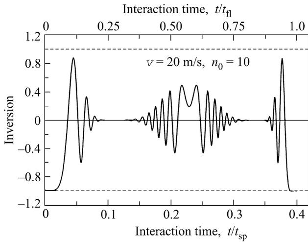
**Fig. 2.** Time evolution of the inverse population of an atom passing with the velocity  $v = 20$  m/s through the cavity with the average number of photons  $\langle n_0 \rangle = 10$  before the atom enters the cavity. The lower time scale is in units of spontaneous lifetime  $\tau_{sp}$  of the excited atomic state. The upper time scale is in units of atomic time of flight through the cavity.
