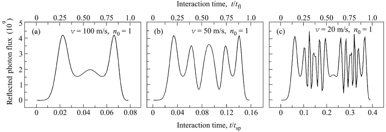
**Fig. 4.** Time dependence of the photon flux reflected from the cavity containing one photon on average ( $\langle n_0 \rangle = 1$ ) and through which the atom passes with the velocities  $v =$  (a) 100, (b) 50, and (c) 20 m/s.
