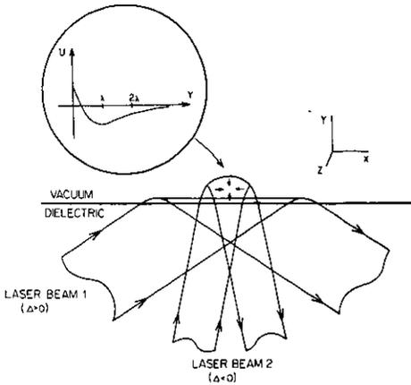
**Figure 1.** Schematic diagram of the evanescent light trap formed by the evanescent waves of two laser beams undergoing total internal reflection at a dielectric–vacuum interface. The curve in the circle shows the atomic potential energy in the trap as a function of the  $y$  coordinate.
